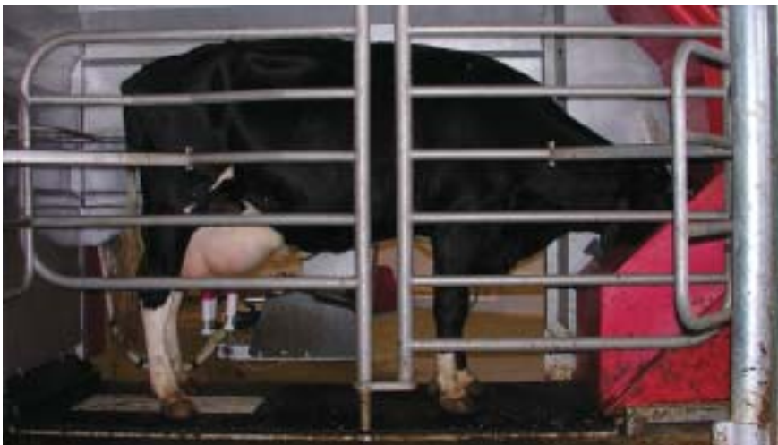
Cows “chase energy” by nature, and voluntary milking relies on the promise of high-energy food treats to entice cows to milking. Sensors read ID tags around the cows’ necks and do not allow them back into the milking stalls until a minimum time has elapsed. Milking intervals are programmed by the farmer. Cows that are rejected by the system return to the pasture and try again later. Each cow has an ID number dyed into her side to allow easy surveillance by the 15 video cameras mounted in the barn. (Photos by Glenn Laing and Sue Mitrovich)
