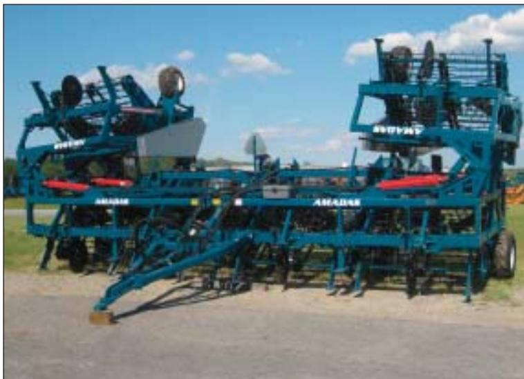
for more efficient use of tractor horsepower. A 220 hp tractor used to carry a conventional 8-row digger is more than sufficient to tow this 12-row model. Not only is the digging efficiency increased, but tractor and operator expense may also be reduced when comparing operation of the ADI-1236PT against a conventional 8-row or two 6-row digger/inverters.
