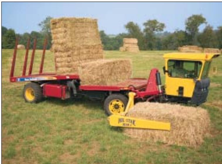
Holland Self-Propelled Balewagon the only product to date capable of handling both small square and large square bales. While the current use for this product is primarily for handling hay products for feeding livestock, future use for handling biomass bales is a major benefit.
