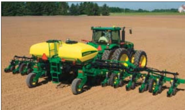
frame design; these wheels reduce the amount of weight placed on the rear of the tractor and support the CCS cradle. This design provides a balanced planter for maneuverability in the field and during transport. 1720 CCS Planters work well in conventional or reduced-tillage field conditions and are ideal for planting into strip-till conditions.
