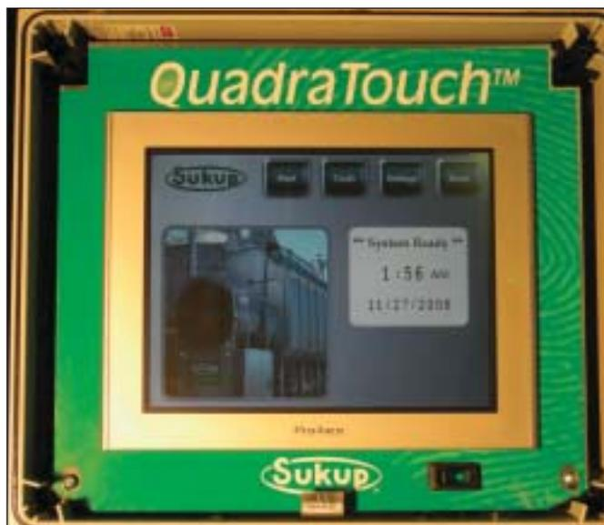
The QuadraTouch™ is a PLC-based system. PLCs are rugged and are built to withstand harsh environments. They offer superior noise protection, eliminating nuisance trips.
