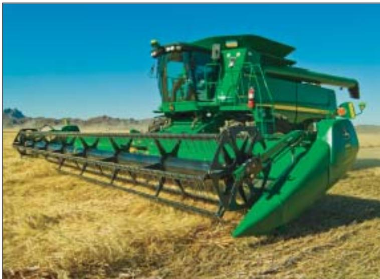
hydraulic cutter bar tilt, ContourMaster™ integration, center drum/center draper belt/reel reverse with feeder house, in-cab belt speed display, reel resume capability, and no-tool/one-person conversion to four-tire transport configuration. The platform is available in three sizes: 7.6, 9.1, and 10.7 m (25, 30, and 35 ft).
