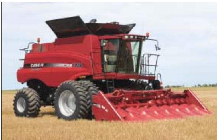
Clean grain elevator capacity has been increased 15 percent, a two-speed header drive is an option, and the 88 Series now shares a common feeder/header interface with the Case IH 20 Series Axial-Flow® models. The all-new styling utilizes body panels made from soy-based sheet molding compound (SMC) material and includes low rear trim panels to keep dust and crop residue from accumulating on the engine deck.
