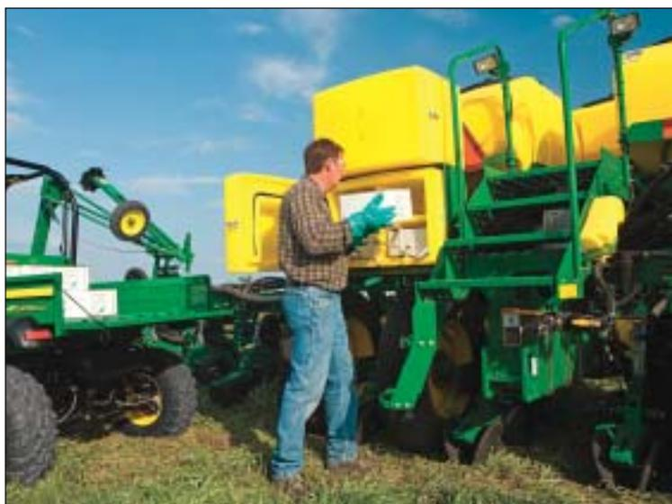
closed calibration procedure at one central location to protect the operator from insecticide exposure. Comparable granular-type insecticide systems require the operator to collect chemical from each row unit on the planter.
