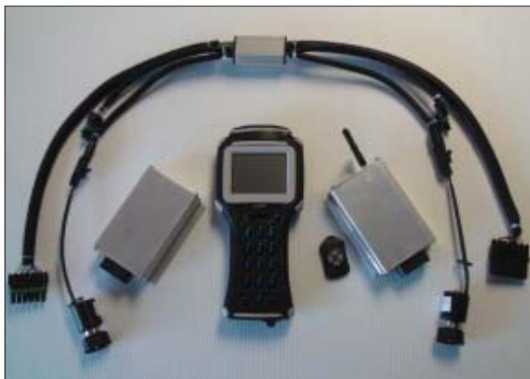
The system also incorporates a wireless interface to control individual nozzles, useful in locating nozzles that are not working properly.
