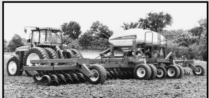
Large central tanks, wide widths, and fast operating speeds mean increased productivity. Standard features include in-cab rate adjustment, accurate seed counting monitor, low level bin sensor, half-width disconnect, and choice of three metering wheels. Optional features include rear auxiliary hydraulic couplers and platform-mounted fill lights.
