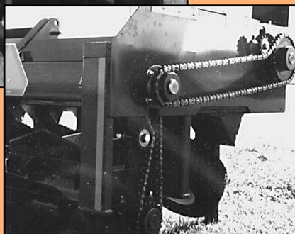
**T**he AMADAS **CSP01 Cotton Stalk Puller/Chopper** is designed to streamline post-harvest cotton stalk management and field preparation. Pulling up an entire cotton stalk and chopping it into small pieces, the CSP01 can perform in a single pass what previously took several machines and three to five passes. Operating at 8 to 12 mph, it is common for this four-row machine to cover 100 acres per day, resulting in time and cost savings. Other benefits include
