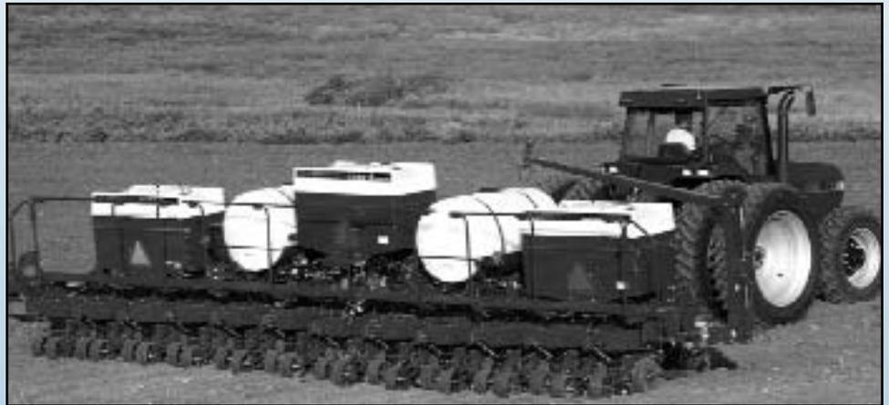
hydraulic pressures, a piston pump for liquid fertilizer delivery and narrow gauge wheels for improved residue flow. **Case Corp.**, Burr Ridge, IL, USA; 630-887-2341.
