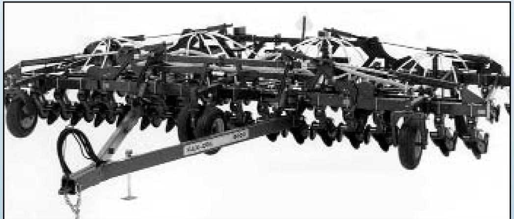
soil with less down pressure. A cleaning wheel keeps soil from moving up and away from the blade, forming a slot for seed placement. A V-shaped press wheel follows the blade, pressing at the opposite angle to completely close the slot, leaving
