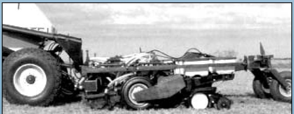
openers on the tool bar. In both cases, a transfer system allows the air cart weight to be hydraulically distributed evenly across the tool bar for penetration control in a variety of soil types. **Flexi-Coil, Saskatoon, Saskatchewan, Canada; 306-934-3500.**
