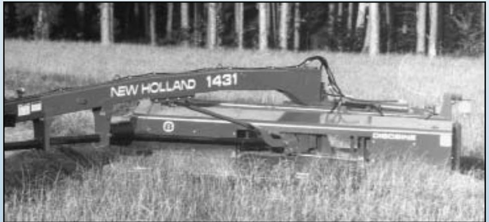
ular discs with a 3.9-m (13-ft.) cutting width and has 2.6-m (102-in.) intermeshing rolls. **New Holland North America, Inc.**, New Holland, PA, USA; 717-355-3656.
