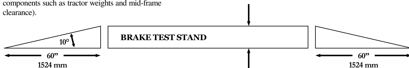
Figure A-8 Approach and Departure Requirements
