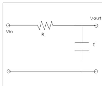
A filter to remove 60 Hz noise from pulses being transmitted at 2,000 Hz for a stepping motor is to be designed. Pulse amplitudes are not to be reduced by more than 3 dB with a critical frequency of 2 Hz in the filter. The voltage attenuation for this high pass filter is most nearly:
