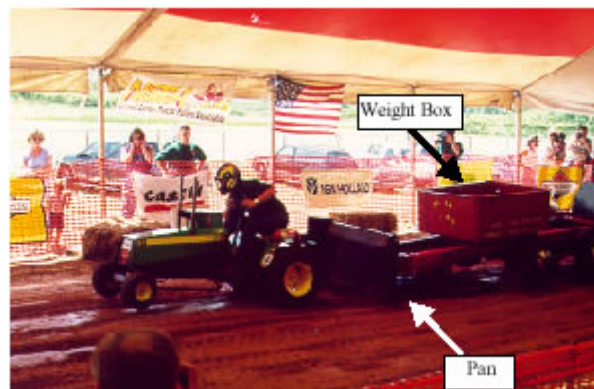
Figure 2a: Typical Progressive Sled in Action.
