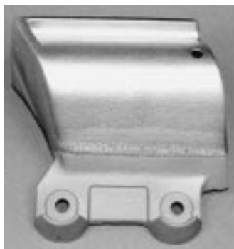
Coated element used in high-productivity STS combine.
