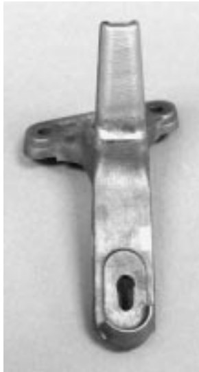
Coated tine used in high-productivity STS combine.
